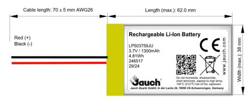
Thickness (max.): 5.4 mm (deliver status) 5.8 mm (after cycling)
