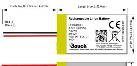
Thickness (max.): 10.0 mm (deliver status) 11.0 mm (after cycling)
