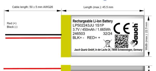
Thickness (max.): 5.4 mm (deliver status) 5.8 mm (after cycling)
