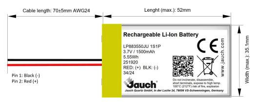
Thickness (max.): 9.0mm (delivery status) 9.72mm (after cycling)
