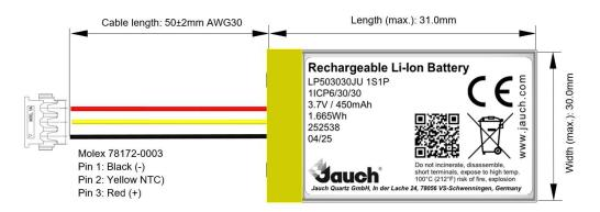
Thickness (max.): 5.2mm (delivery status) 5.6mm (after cycling)
