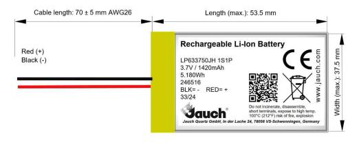
Thickness (max.): 6.3 mm (deliver status) 6.8 mm (after cycling)
